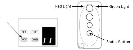
c) Press the same button on transmitter again, the dot(.) on the display will flash, now you have finished the coding.
